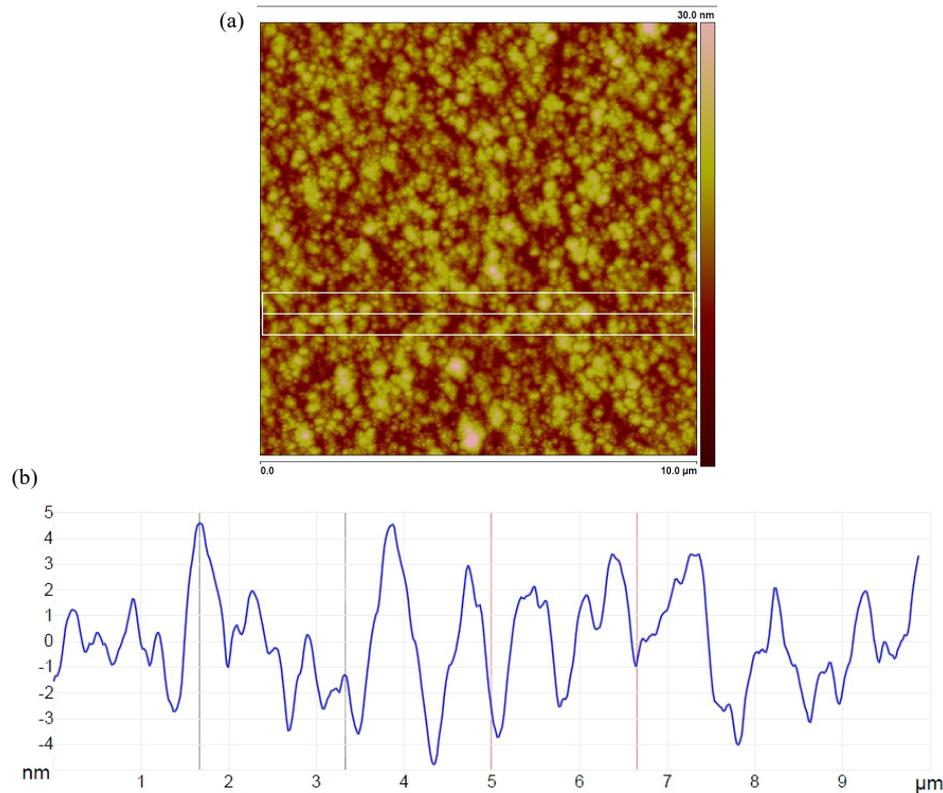
**Fig. 3.** AFM image of a surface fragment of an epitaxial gallium oxide layer grown on a bulk gallium oxide substrate: (a) surface map, (b) profile along the marked line.
