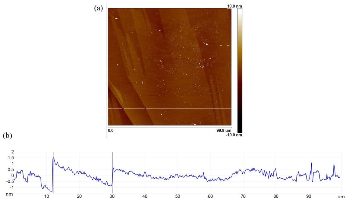
**Fig. 1.** AFM image of the substrate surface: a) surface map, b) roughness profile along the marked line.
